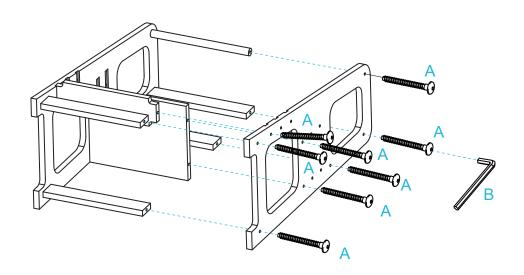
Attach all panels together as shown and secure with 8 x bolts (A). Tighten with an Allen Key (B).
